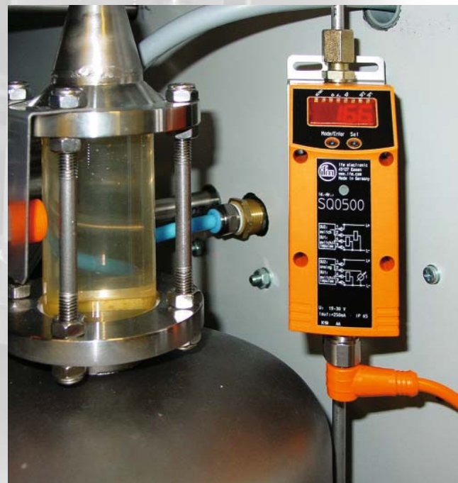
Sensor for the measurement of smallest dosing quantities.
